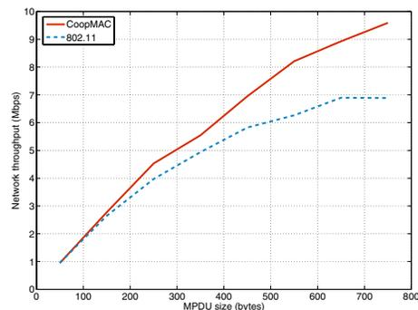
Fig. 4: Throughput comparison as the MPDU size increases
