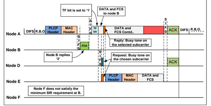
Fig. 4: Source based three node FD transmission.
