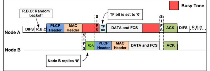
Fig. 2: Two node FD transmission.
