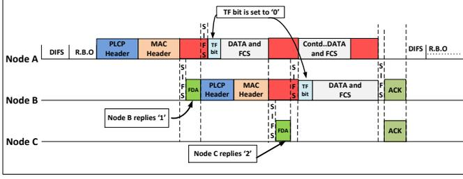
Fig. 3: Destination based three node FD transmission.
