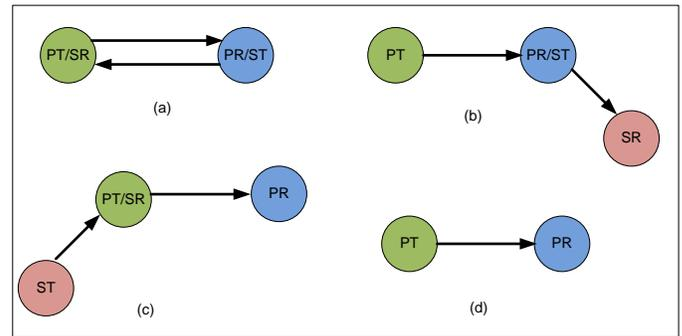
Fig. 1: Different scenarios of exploiting FD capability, (a) Two node FD transmission, (b) Destination based three node FD transmission, (c) Source based three node FD transmission, (d) HD transmission.
