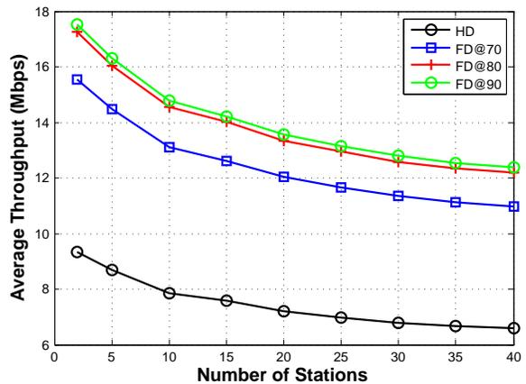
Fig. 5: Throughput as a function of number of stations for different self-interference cancellation levels (FD@ $x$  means the FD node is capable of canceling self-interference by  $x$  dB).
