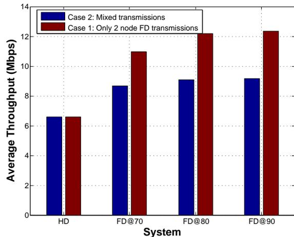
Fig. 6: Throughput for mixed FD (both two node and three node FD transmissions) and only two node FD transmissions for different self-interference cancellation levels (FD@ $x$  means the FD node is capable of canceling self-interference by  $x$  dB).
