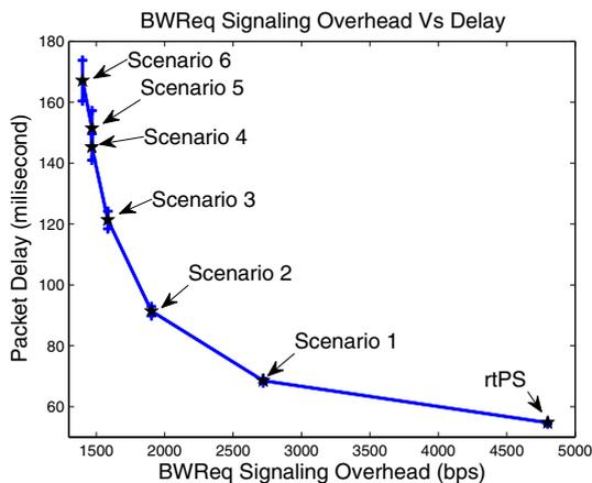
Fig. 6. Online gaming: packet delay vs. *BWReq* signaling overhead.
