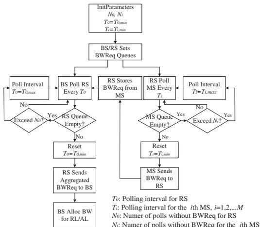
Fig. 4. The Proposed Bandwidth Request Algorithm (mPS) in WiMAX.
