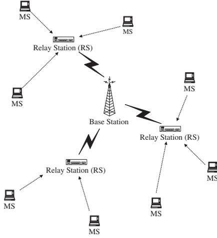
Fig. 2. The Centralized Multi-hop WiMAX Network.
