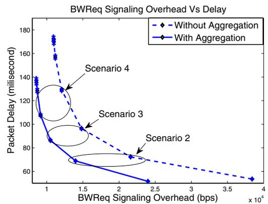
Fig. 7. Online Game with aggregation: Delay vs. *BWReq* signaling overhead.
