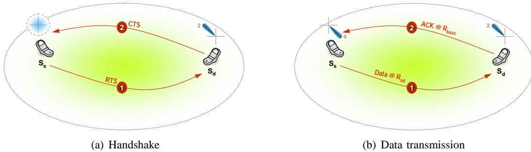
Fig. 2: Illustration of the proposed directional non-cooperative MAC (D-NoopMAC).
