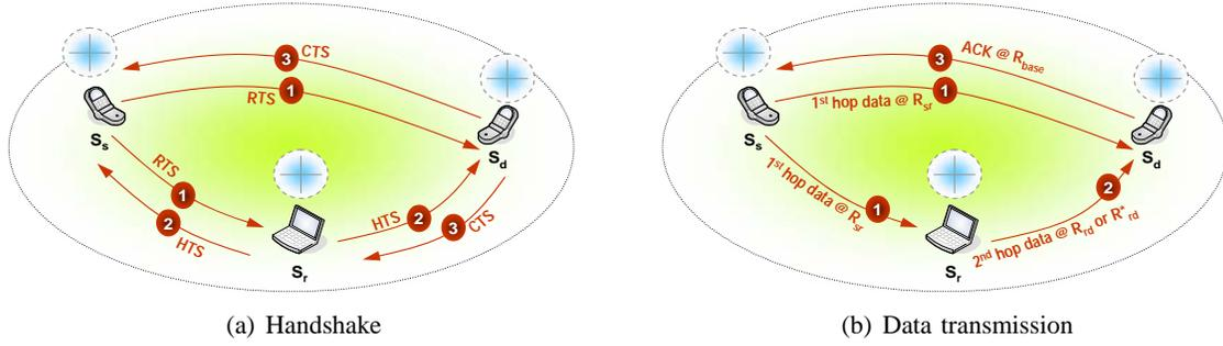
Fig. 1: Illustration of the proposed cooperative MAC with omnidirectional antenna (O-CoopMAC).
