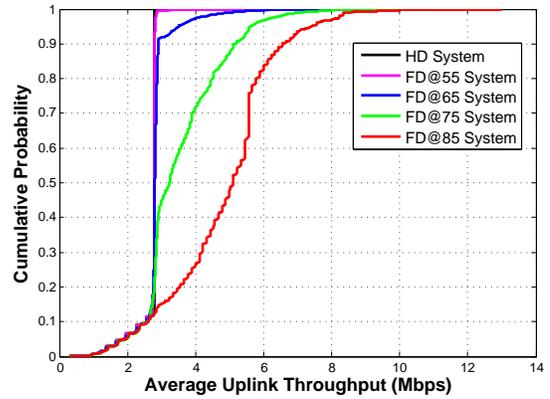
Fig. 7: Distribution average data rates in uplink.
