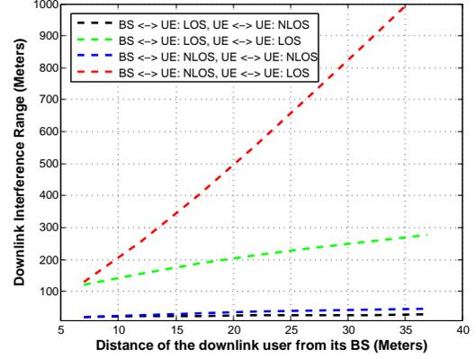
Fig. 4: Downlink interference range with different channel conditions ( $P_{BS} = 1.78$  dBm, and  $P_{UE} = 0.78$  dBm).
