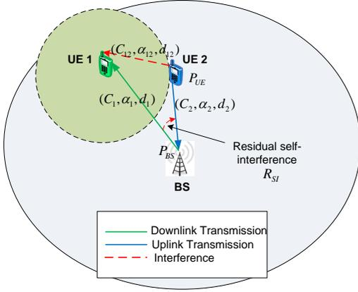
Fig. 3: A full-duplex small cell showing the interference range.
