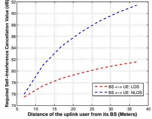
Fig. 5: Minimum required self-interference with different channel conditions ( $P_{BS} = 1.78$  dBm, and  $P_{UE} = 0.78$  dBm).
