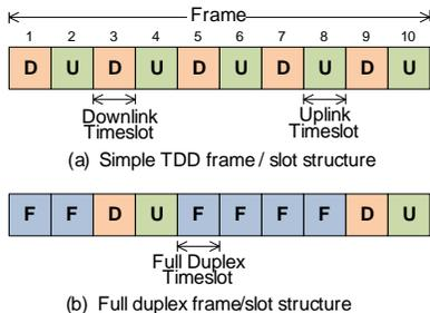
Fig. 1: TDD half duplex baseline and full duplex operation.
