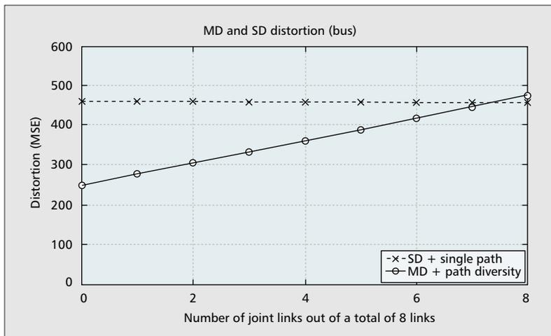
■ **Figure 3** MD vs. SD distortion as the number of joint links between two paths varies. Simulation parameters are given in [4].
