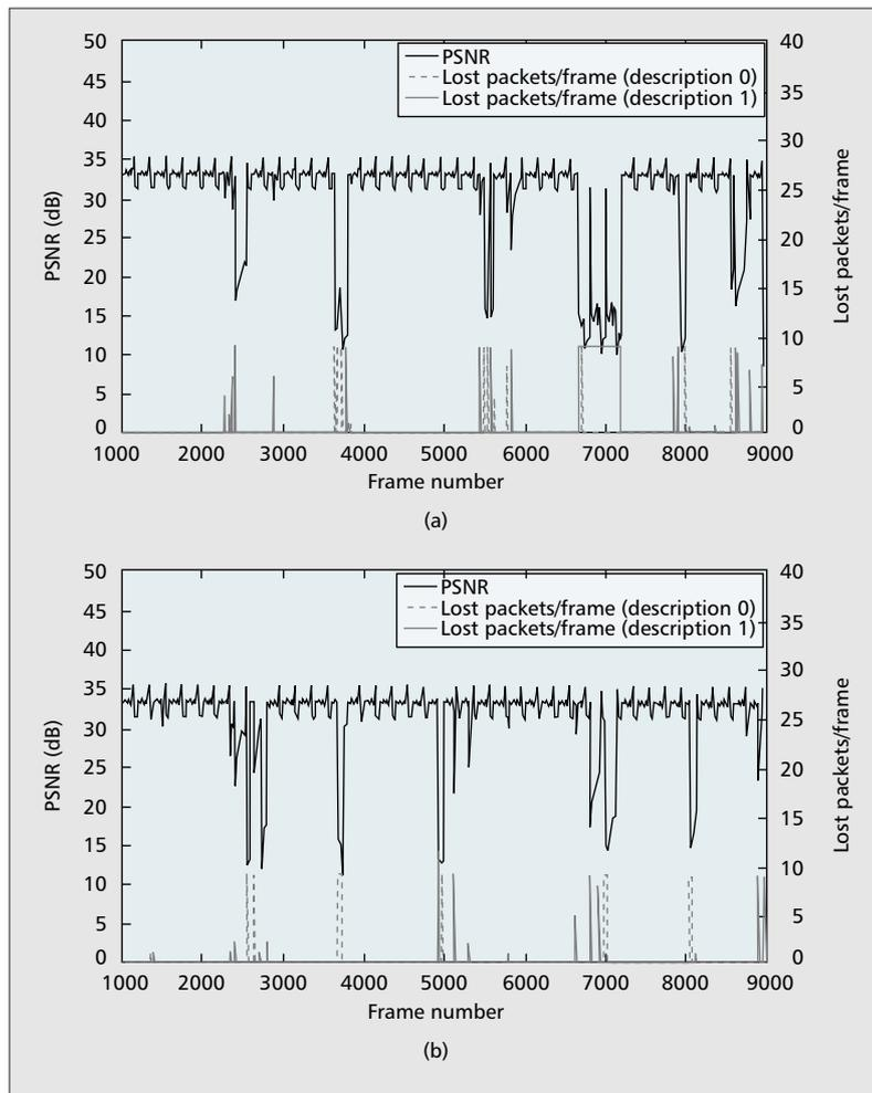
**Figure 5.** Comparison of a) single path transport; b) multipath transport (two paths used). The top curve in each figure shows the PSNRs of received frames; the lower curves show the packet losses per frame experienced by the two streams. The average PSNR is a) 30.19 dB; b) 31.45 dB.
