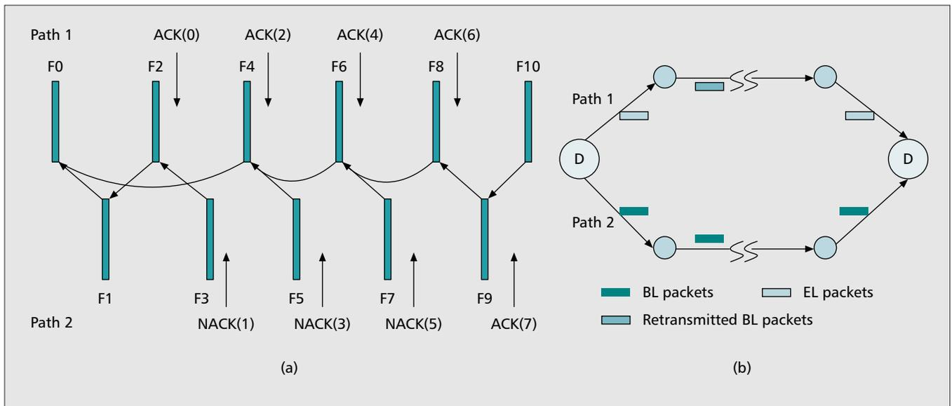
■ **Figure 2.** a) The RPS scheme: the arrow from a frame indicates the reference picture used in coding that frame; b) the two-path layered video transmission model with selective ARQ for base layer packets.
