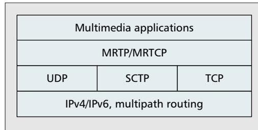
■ Figure 4. The protocol stack using MRTP.
