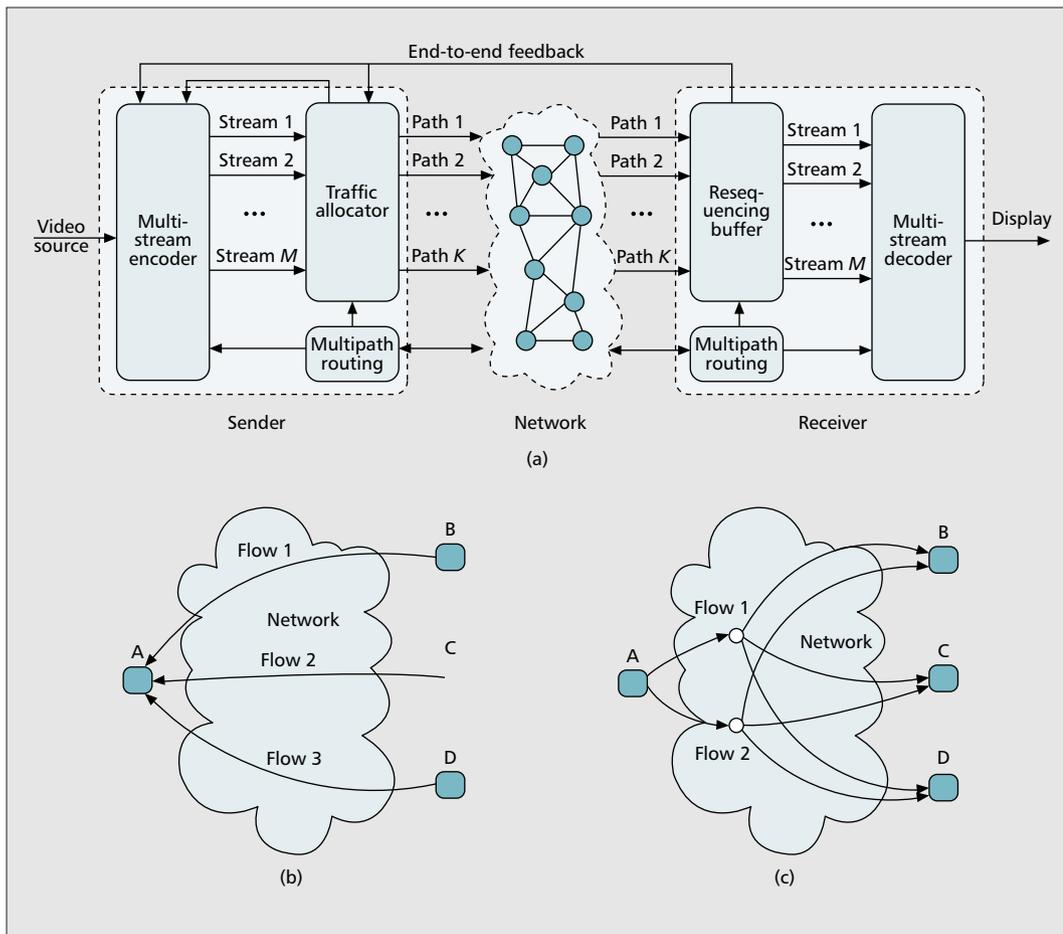
■ **Figure 1.** The general architecture for the multipath transport of realtime multimedia applications: a) point-to-point video communications; b) concurrent streaming; c) multicast using two trees.
