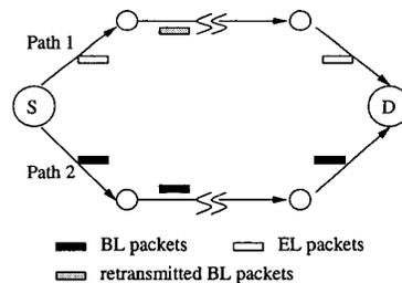
Fig. 3. The two-path layered video transmission model with end-to-end ARQ for BL packets
