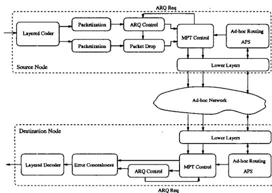
Fig. 1. An architecture for layered video transmission over ad-hoc networks using ARQ and MPT
