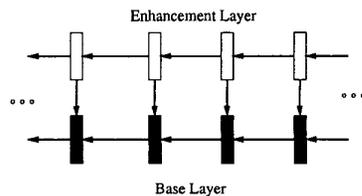
Fig. 2. The layered coding scheme
