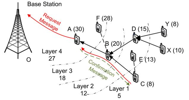
Fig. 2. Greedy Helper Discovery Protocol and Routing Protocol. The numbers in parenthesis are the average 3G rates for each node. The dashed line indicates the ad-hoc neighborhood. The straight solid line is the ad-hoc path with the arrow pointing to the helper. For routing protocol, dashed-dotted lines represent the coverage area of each layer. 27, 18, 12 and 5 are the physical transmission rates for layers 4, 3, 2 and 1.
