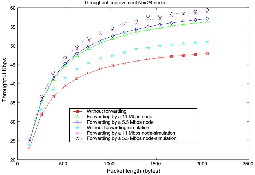
Figure 6. Throughput vs packet length.
